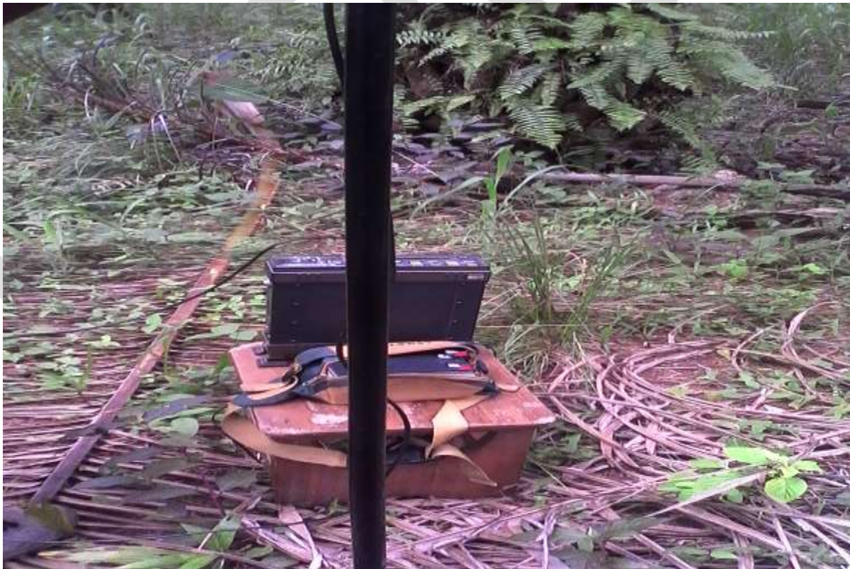
Appendix 3: Picture of campaign in one of the forested site with the CATV (cable) Analyzer, its charger and the receiver antenna pole
