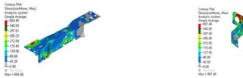
Fig 7 Stress plot for side member & Z bracket (Iteration 1)
