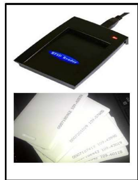
Fig 6: Prototype-RFID Reader and Cards
