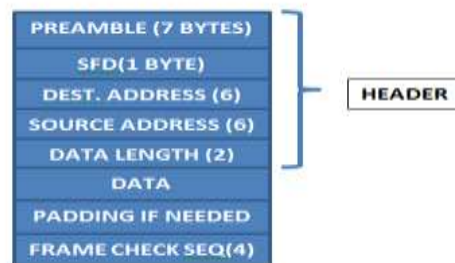
Fig 2: Gigabit Ethernet frame.
